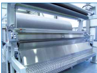
Double station unwinder by Somatec with automatic ultrasonic splicing unit
